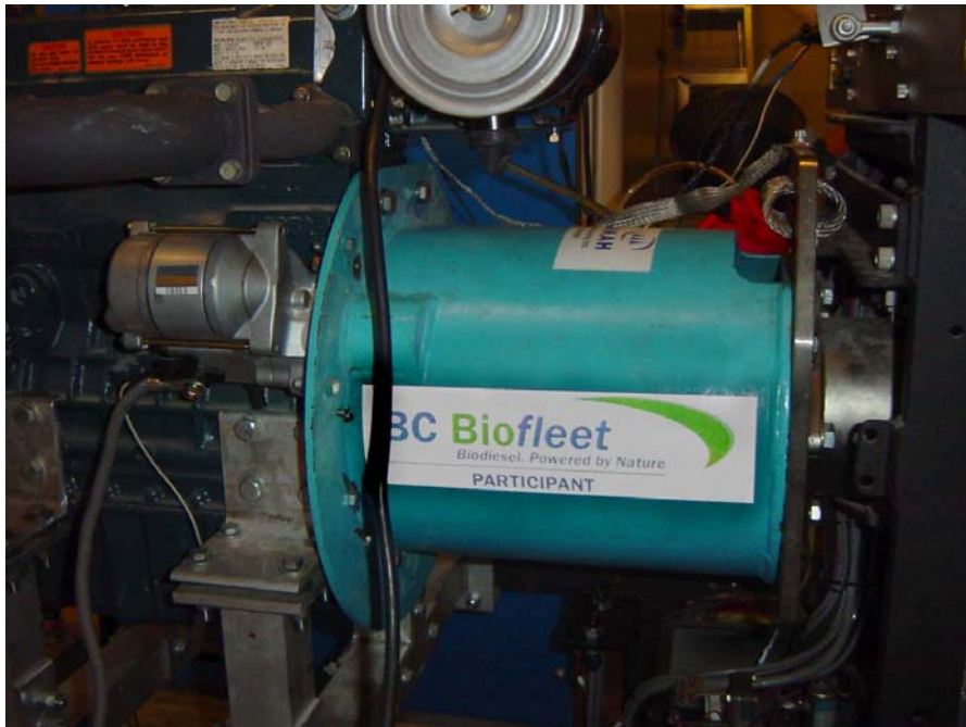
Figure 1: Bell Housing Installed
