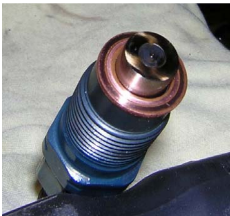
Figure 9: Fuel Injector Tip Before Testing.
